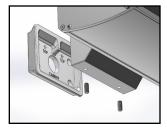
1. Unscrew 3/8"-16 X 7/8" Set Screws and remove the Wall Mount Plate.
