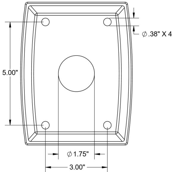
2. Attach wall mount plate to wall with (4x) hex nuts and washers (not included).
