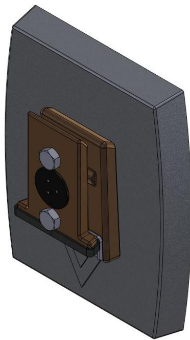
5. Place wall mount cover on wall mount plate and tighten (2x) screws at the bottom of wall mount cover.
