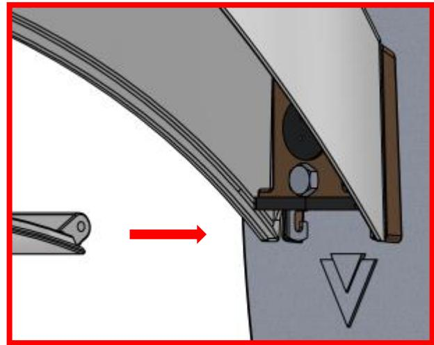
8. Attach door to the security cable assembly and push it up to close the luminaire.
