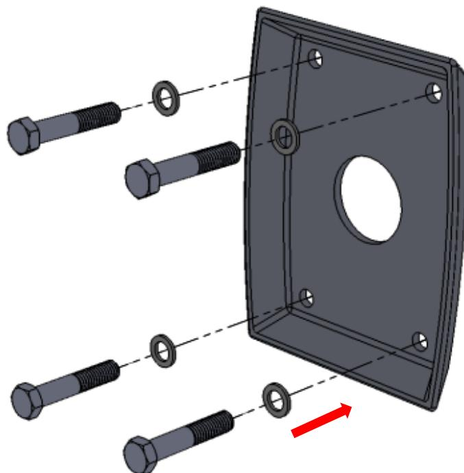
3. Align (2x) screws with castings provisions, wall mount cover, nut plate and nuts.
