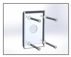
1. Install Wall Mount Plate to the wall with washers and bolts (by others). Make sure it is levelled.
