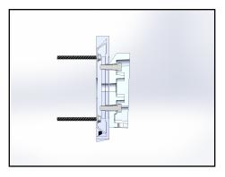
3. Hang the Wall Mounting Casting/BOA Mount Casting Assembly onto Wall Mounting Plate. Secure in place by tightening 3/8"-16 Set Screws. Tighten to 20 ft-lb.
