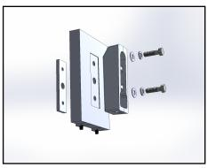
2. Align the holes in the Bolster Plate, Wall Mount Casting and BOA Mount Casting. Secure in place with 1/2" Flat Washers, Split Lock Washers and Hex Bolts. Tighten to 30 ft-lb.
