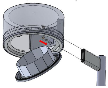
**5.** Align (1X) latch to door provision. Turn right the latch (1X) to close the door.
