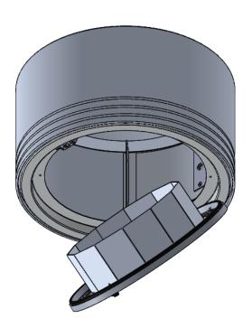
**4.** Align (2X) threaded rods, CON-2-L housing provisions, (2X) flat washers, (2X) lock washers and (2X) hex nuts. Fasten the components to secure CON-2-L housing to bolt on arm.
