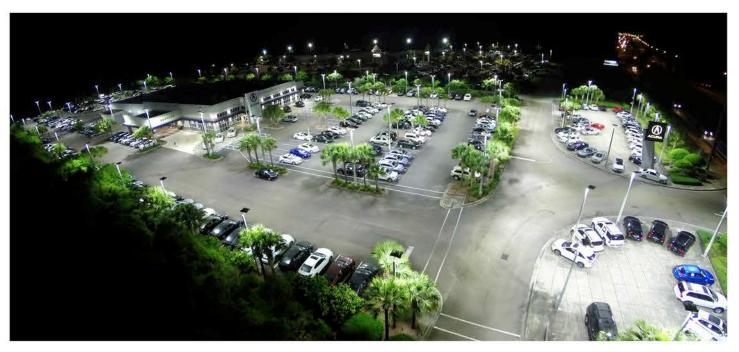
Summary - Replaced with BLX-III fixtures - 55% fixture count reduction Reduced wattage by 74%
