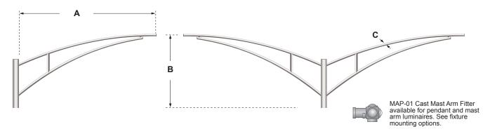
**VA114** is constructed of 2% Ø extruded aluminum tubing, designed for Roadway applications. **VA114** is designed to slip over the following tenon (or pole) sizes: 3" Ø,  $3\frac{1}{2}$ " Ø, 4" Ø and  $4\frac{1}{2}$ " Ø. **VA114** is available in the following pole mounting configurations: Single and Double 180°. Please consult factory for custom mounting.
