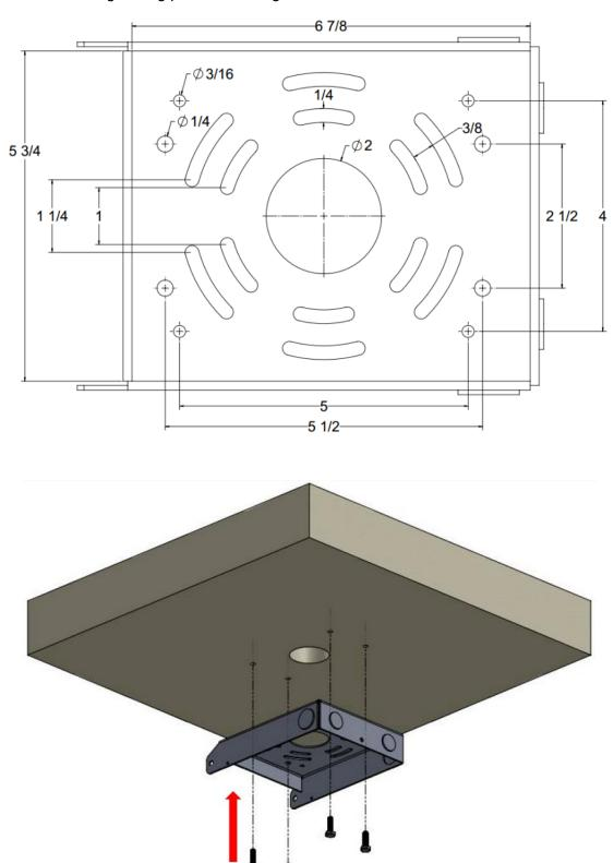
4. Route electrical wires from fixture (marked in blue) through mounting plate hole (marked in green) to connect to power supply.
