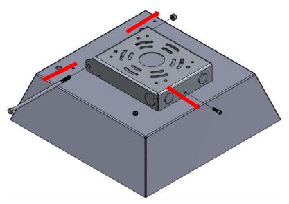
2. Disassemble mounting plate from bottom bracket.
