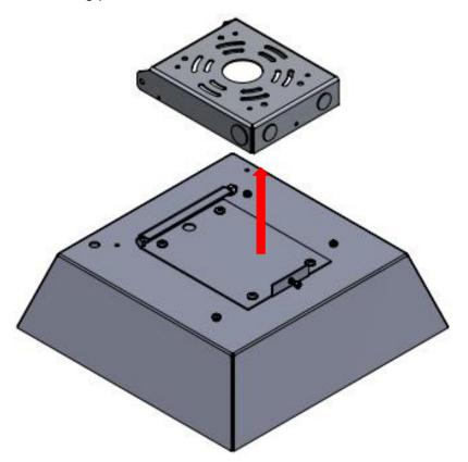
3. Secure mounting plate to ceiling junction box using hardware of your choice. Please refer to the following drilling pattern drawing.
