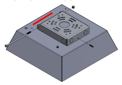
6. Align (X1) screw sockets head cap and ceiling mount bracket. Fasten (X1) screw socket head cap.
