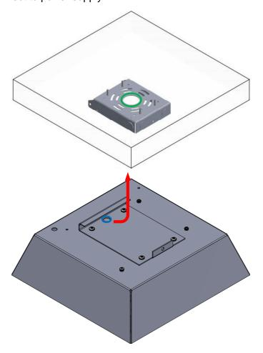
5. Align (X1) hex head cap screw partial thread, ceiling mount brackets and (X1) nut. Fasten (X1) hex head cap screw partial thread and (X1) nut.
