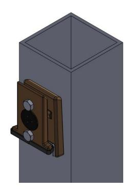
3. Slide luminaire Driver Compartment between the Castings and Fasten tightly (2x) screws.
