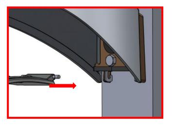
**5.** Attach Door to the Security cable Assembly and push it up and turn the tumb screw to close the luminaire.
