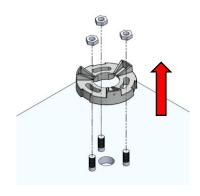
4. Install the Vandal-Resistant Base (VRB) with the nuts I removed earlier.
