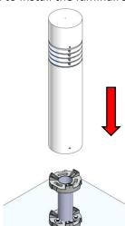
6. Screw in luminaire with the screws you removed earlier.
