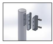
1. Align the holes in the Pole Bolster Plate, Round Pole Adapter (wide end toward the top of the pole), BOA Mount Casting and Pole, and secure in place with 1/2" Flat Washers and 1/2"-13 X 2-1/4" Thread Locking Hex Head Bolts. Tighten to 30 ft-lb.
