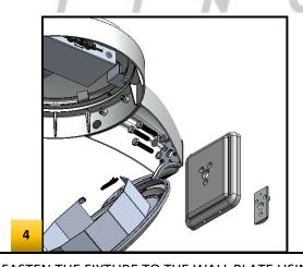
FASTEN THE FIXTURE TO THE WALL PLATE USING THE  $\frac{1}{2}$ -13 x 2 "LONG SCREWS AND THE NUT PLATE.
