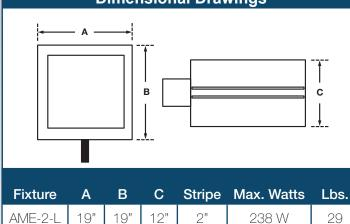
The new American LED Luminaire from Visionaire combines contemporary design with new LED technology; while maintaining a traditional fixture image. The LEDs Performance and Life are maximized by the unique integral aluminum heat sink built into the door frame. Maintenance of the drivers is simplified by making them easily accessible and provided with quick wiring connections.
