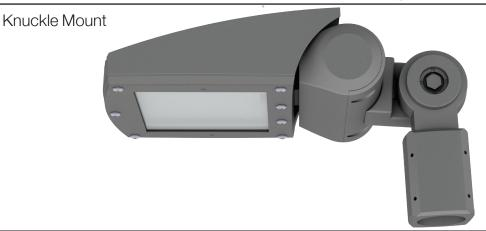
An adjustable knuckle slip fits over a 2-3/8" Tenon, and allows for up to 90 degrees of vertical adjustment in 10 degree increments from horizontal, as well as full side to side adjustment with the knuckle mount.
