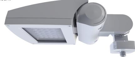
An adjustable knuckle slip threads over a ¾" NPT, and allows for up to 90 degrees of vertical adjustment in 10 degree increments from horizontal.
