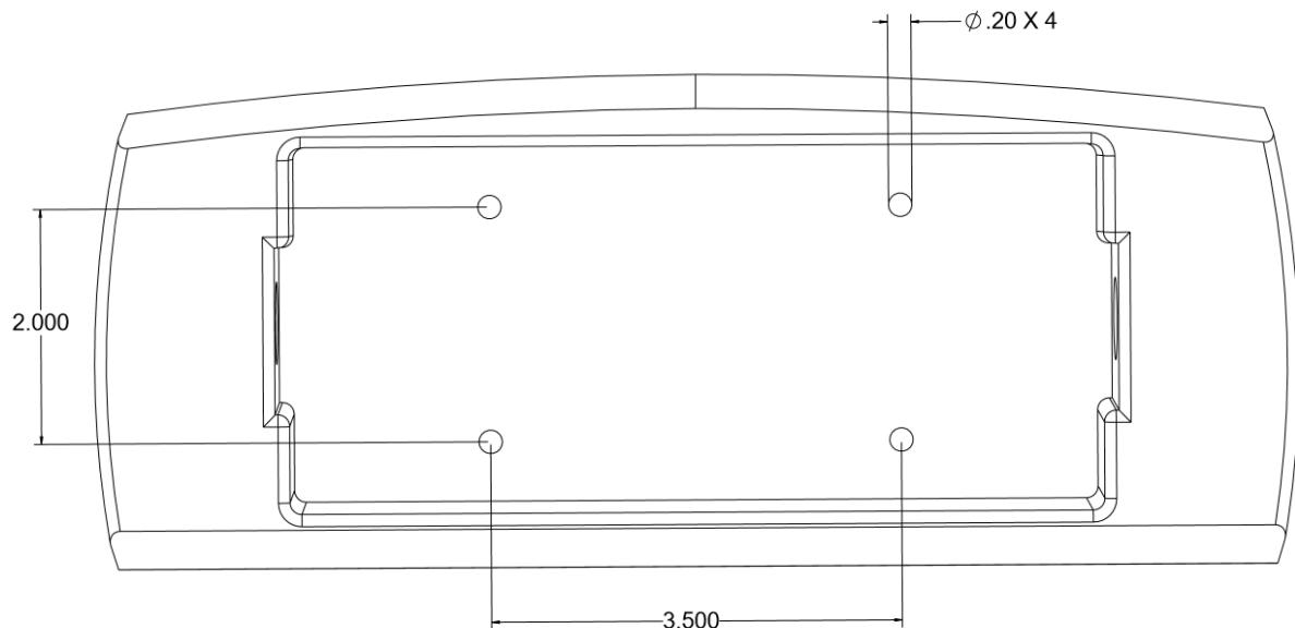
2. Attach wall mount plate to wall with (2x) hex nuts and washers (not included).
