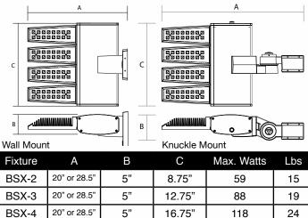
The new BOW SX LED Series continues the unique contemporary design inspired by the sleek styling of the BOW family. Separating the extruded aluminum driver housing and the individual die-cast aluminum linear LED engines: optimize the life of the LEDs and the Driver(s); and maximizes the lumen output of the fixture.
