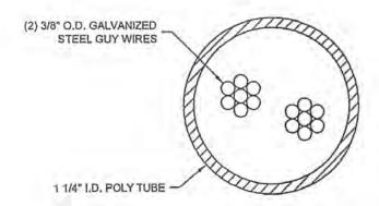
VIBRATION DAMPENER CROSS SECTION
