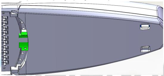
1. Loosen the four1/2"-13 hex head bolts holding the two clamps brackets enough to slide lamp into arm aprox 4.5" (125mm) deep, until arm rest on steps that would sit between the mast arm and pipe clamps and run electrical feed wires to inside of lamp terminal block.
