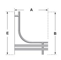
The **VA105-L** dimensions are for standard size 2 or size 3 Architectural luminaires only. **VA105-S** is standard for smaller, size 1 luminaires.
