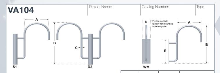
The **VA104-L** dimensions are for standard size 2 or size 3 Architectural luminaires only. **VA104-S** is standard for smaller, size 1 luminaires. Center section of arm will match pole design (i.e. fluted pole = fluted center arm section).
