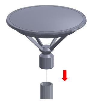
**3.** Fasten (x6) set screws to secure in place.
