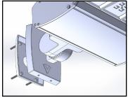
4. Secure BLX-II luminaire in place by tightening the 1/4" Set Screws to 7 ft-lb.
